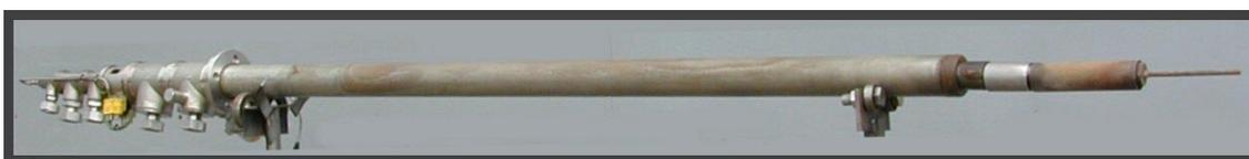
Figure 4. A specific deposit-monitoring probe can be applied in analysing both short- and long-term deposition build-up.
