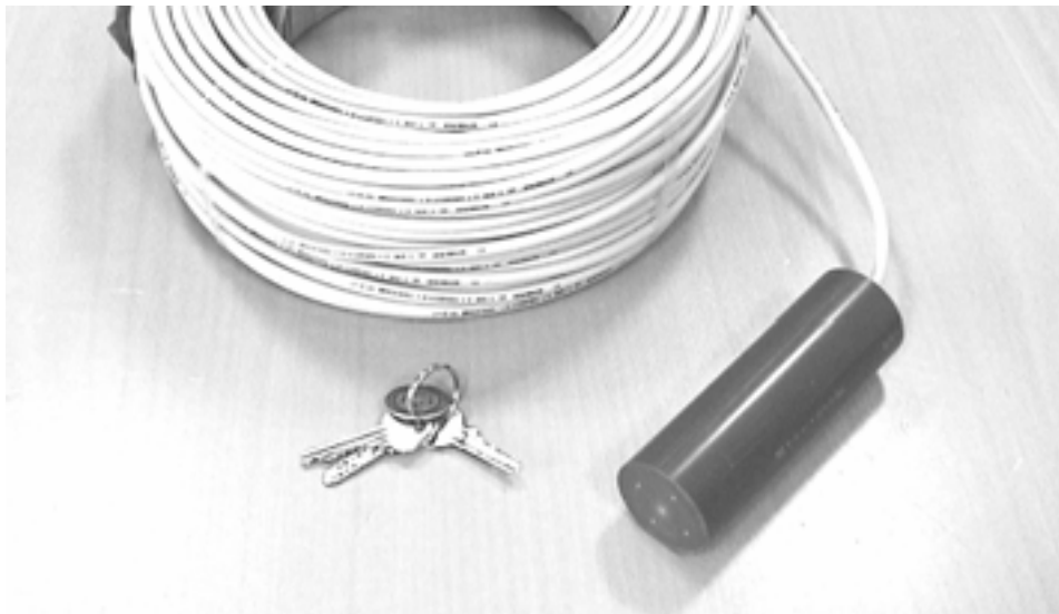
Figure 3-10: Photograph of reservoir water resistivity and temperature probe. The electrodes are visible on the bottom of the probe, while a temperature sensor is placed inside the cylinder, which also houses a lead weight and is filled with polyurethane mould.
