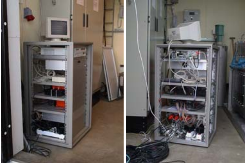
Figure 3-8: Photographs of data acquisition system mounted in 19" rack cabinet: Left: in operation with side panel removed, Right: rear view with electrode cables etc. connected.
