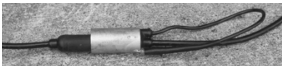
Figure 2-4: Electrode mounted on multi-core cable used on the upstream side.
