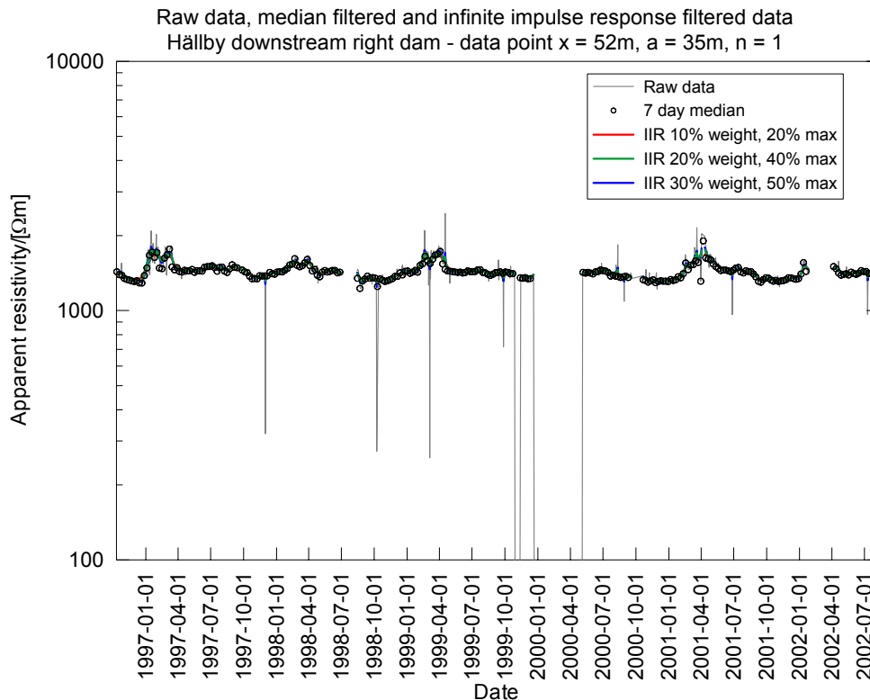
Figure 6-9: Apparent resistivity vs. time measured with 35 m a-spacing Wenner array with midpoint at section 52 m downstream Hällby right dam.
