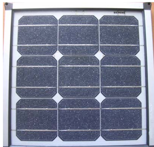
Figure 2. The Siemens reference cell that was used for measuring irradiance and cell temperature.
