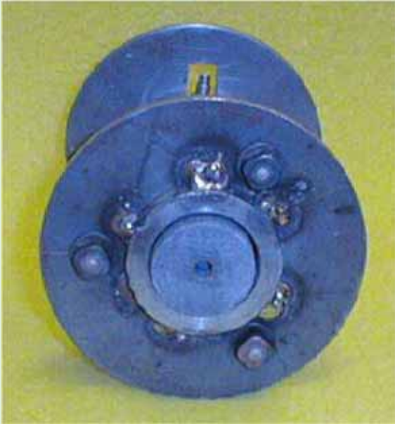
Central spring loaded geophone Force transmitted through tube
