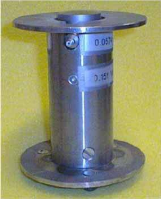
Force transducer and velocity transducer (geophone)
