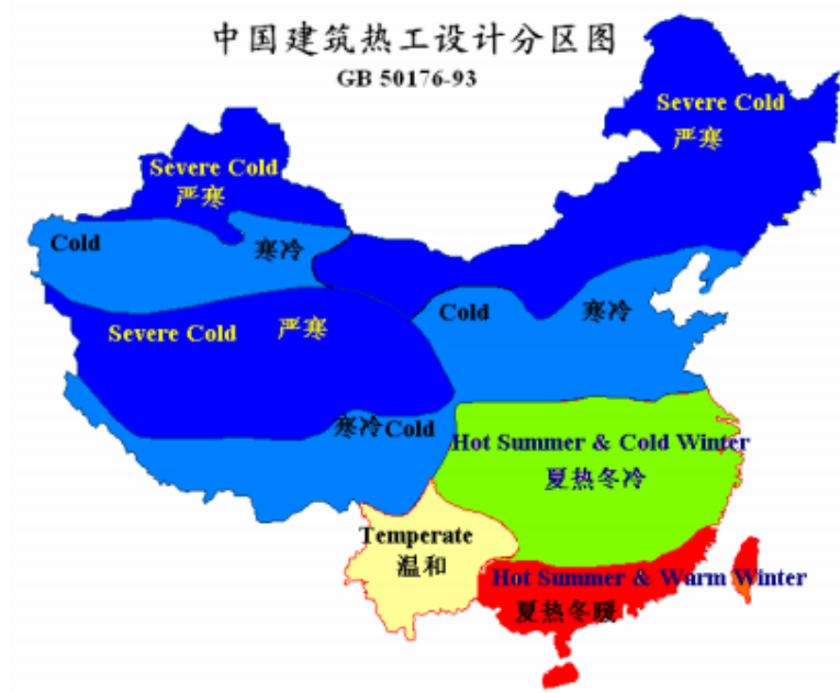
Figure 4.3. Map showing the various Chinese climate zones defined by the Ministry of Construction. Map from (Draugelis, 2011).
