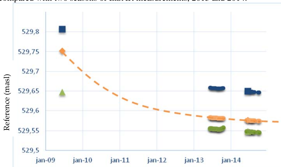
Figure 17. Deformation bolt measurements in 2009 and 2014 (start of 2014 InSAR measurements) of N11, N17 and N14 compared with the relevant InSAR measurement series in 2013 and 2014.
