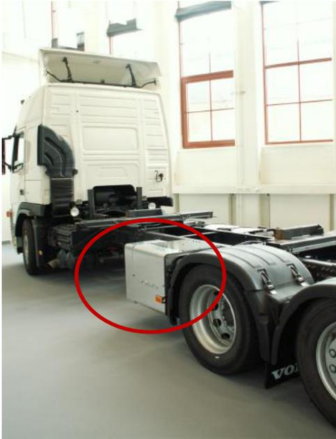
SOFC-APU can operate on diesel
