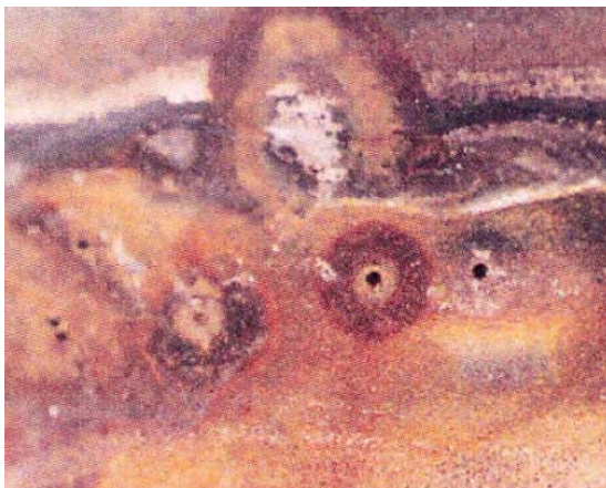
Fig. 8 Pitting sett från angripen yta [8] Fig 8 Pitting seen from attacked surface [8]
