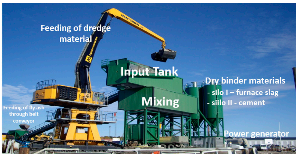
Figur 2.2 Processtabilisering i Åbo. EU Life-Project Stable (Life 06 ENV/FIN/195) Process stabilization in the port of Åbo. EU Life-Project Stable. (Life 06 ENV/FIN/195.)
